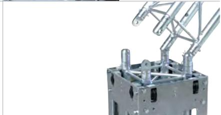
**5** Unscrew the screw jacks in the outriggers. Make sure that the castors of the base are free of any load. The complete load of the base should be supported by the screw jacks. Level the base by adjusting the screw jacks. The base must be perfectly level before the mast is erected. Long outriggers are needed for structures with three towers or less. Make sure the screw jacks can absorb tower forces trough filler plates where needed.
