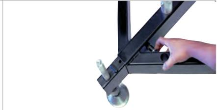
**3** Disassemble the hinge set, mount the half hinges to both the mast sections (H30V truss). Male and female connections should be mounted diagonally (as shown in the picture) in order to facilitate the erection of the mast.
