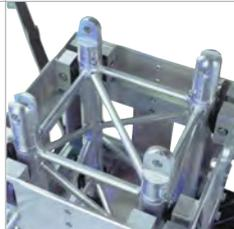
**4** A completely mounted hinge set. First locate the hinge pins on one side. The truss now works as a hinge and can be erected easily. Subsequently locate the remaining hinge pins in the other side to fix the mast into position. Per tower 4 x CCS6-H needed. (hinge set MPT•ST tower).
